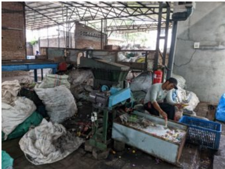
Shredder Machine operator do not wear any PPE
